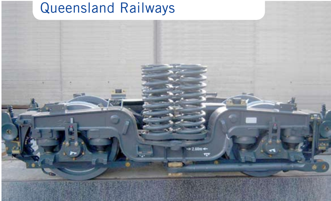
Motor bogie for narrow gauge (1067 mm) with lateral mounted traction transmission for the six-axle locomotive of type QR 3800
