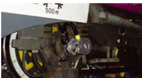
Measuring wheel set for the measuring of the wheel-rail-force during running dynamics type test
