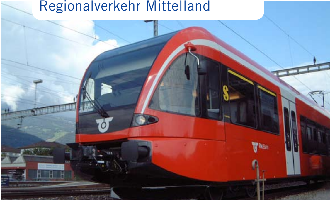
LRV for Regionalverkehr Mittelland between two measuring runs for the running dynamic type test in the station of Sargans
