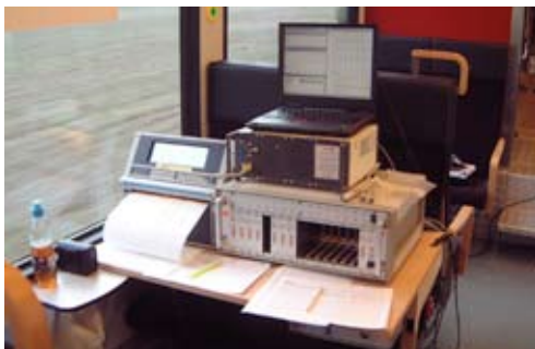
The measuring equipment for recording and online limit value monitoring
