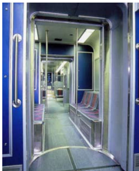
Interior view of the articulation section
