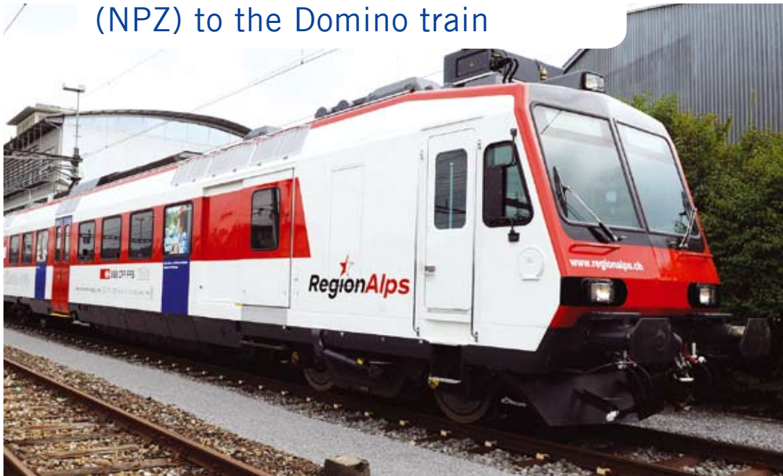
Domino motor coach for the SBB subsidiary Region Alps. Prominent eye catchers are the air conditioning units on the roof. While they enhance the comfort, their integration also presents a technical challenge.
