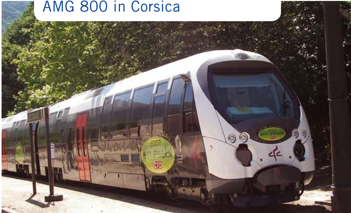
Narrow gauge DMU AMG 800 during type testing on the Corse meter-gauge network
