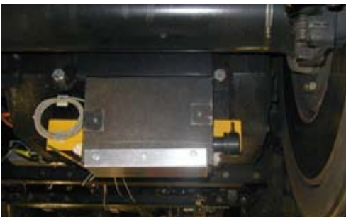
Contactless measurement of the temperature on a wheel brake disc of the NSB EMU Class 72
