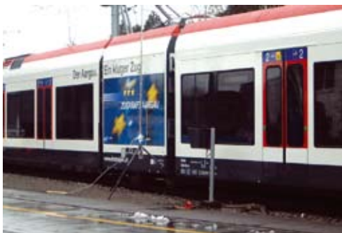
Test of the noise dispersion in original circumstances to be used as a basis for the design of the silencer
