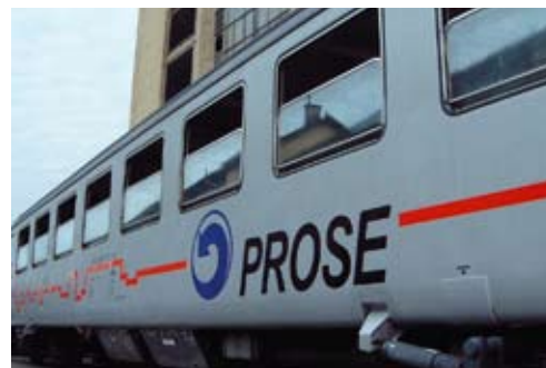
The PROSE measuring coach is based on a RIC passenger coach
