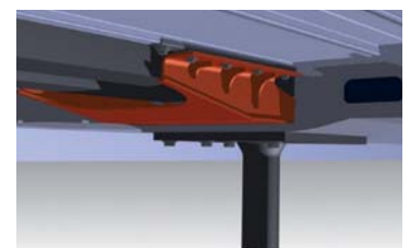
CAD-model of the steel adapter to reinforce the carbody bolster beam
