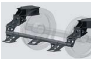
Concept, design, test and manufacturing of 46 new antenna supports on the bogies of the MTRC Lantau Island Airport trains.
