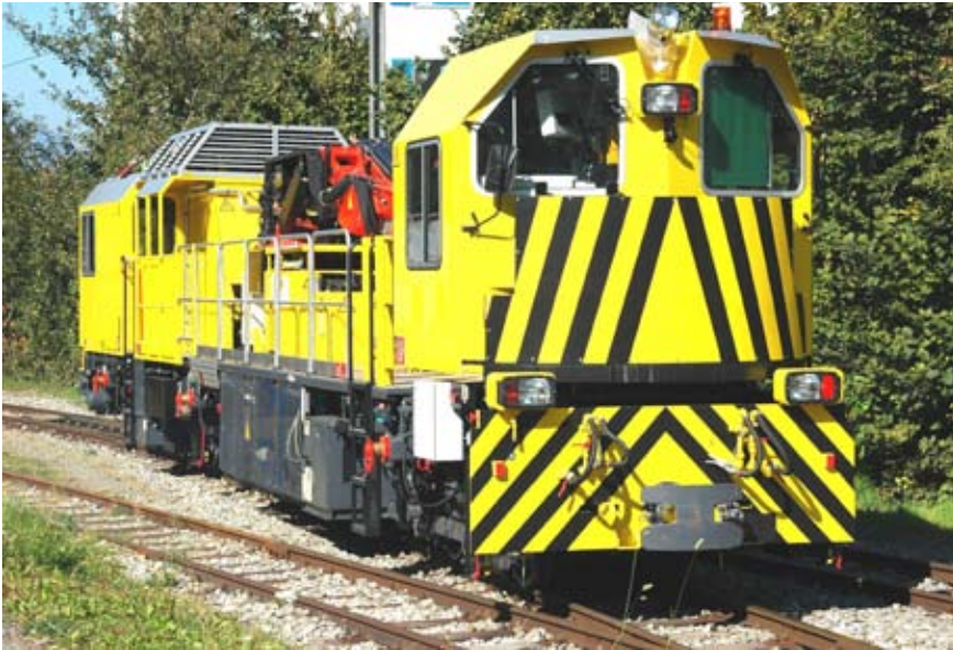
Overhead-line construction vehicle, Plasser-Thurer
