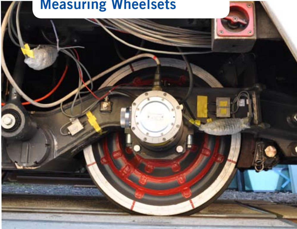
PROSE single measuring wheels PRO03A/B mounted into the PROSE bogie MOB EV 09 during test runs between Montreux and Zweisimmen
