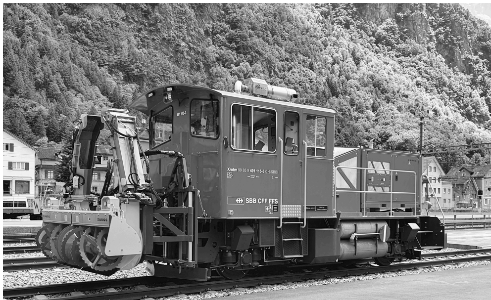
Snow blower Xrotm by SBB and Zaugg, operated by SBB (photo: Stefan Bühler)
