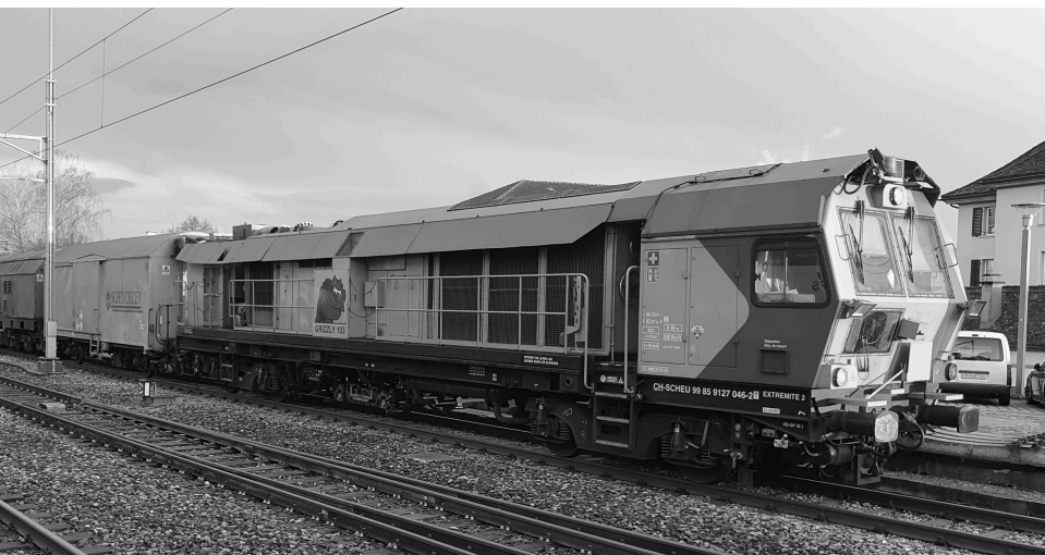
Rail grinding train Grizzly 103 by Scheuchzer, operated by Scheuchzer (Photo: Stefan Bühler)
